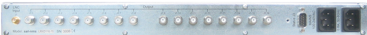
Rear panel view of LRXD116-75 with 1 SMA-type input connectors and 16 F-type output connectors
