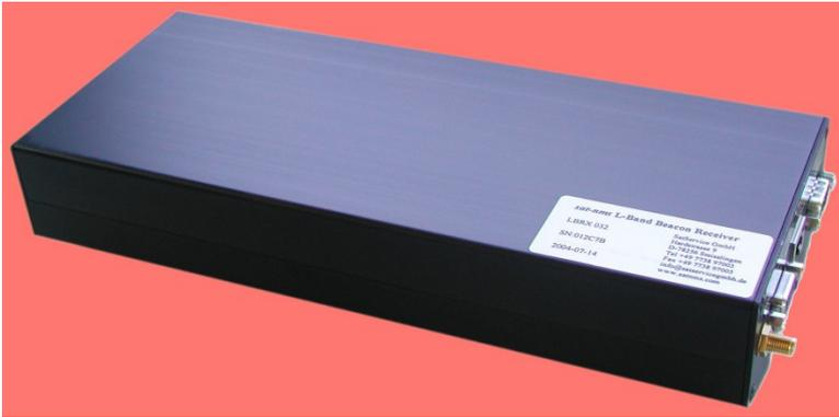
The **sat-nms** LBRX-1MT receives a satellite beacon signal that is down-converted to L-Band via a PLL stabilized Low Noise Converter (LNC) at its L-Band interface input. The **sat-nms** LBRX-1MT does not demodulate any satellite signals because the satellite signals are sometimes CW signals but even more often modulated in FM or QPSK/8PSK form. Due to this fact, the best implementation is a non-coherent receiver that measures the input level in a user selectable defined bandwidth and provides
