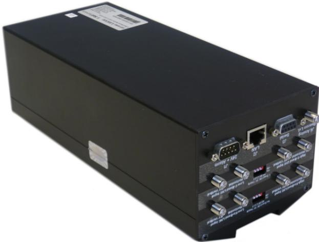
The **sat-nms** LBRX-81 receives a satellite beacon signal that is down-converted to L-Band by a PLL stabilized Low Noise Converter (LNB) at its L-Band interface input. The **sat-nms** LBRX-81 does not demodulate any satellite signals because the satellite signals are not always CW signals but even more often modulated in FM or QPSK. Due to this fact, the best implementation is a non-coherent receiver that measures
