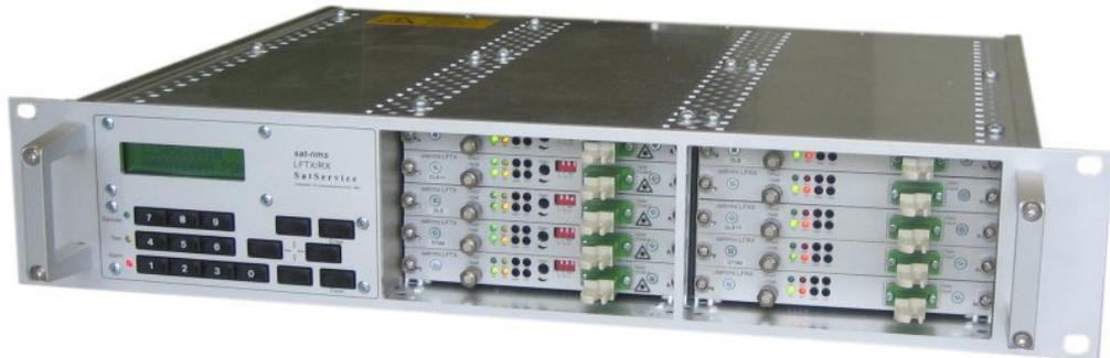
All modules include RF gain adjustment and extensive monitoring. The 19" rack-mount chassis also provides an LCD Display and keyboard for local MNC. The remote MNC interface is via web-browser, SNMP, HTTP GET functions and RS232 interface as in all other **sat-nms** products.
