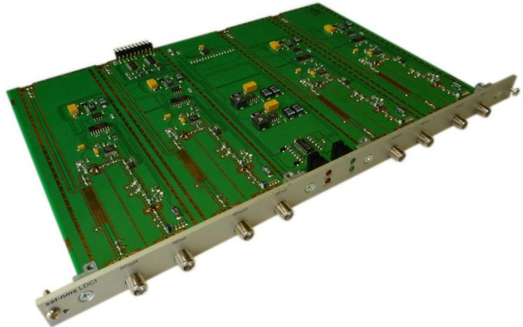
The scalable system is able to support even a single antenna sub-system with 4 LNCs for a small application to a reasonable price, but is also able to provide power to an unlimited number of antennas with multiple **sat-nms** LDCI / MPC chassis. The only restriction is the supply current to the LNBs of max. 5.5 Amps. in total per standard chassis. But the **sat-nms** LDCI can also be delivered in other configurations with the ability to supply a higher total current.
