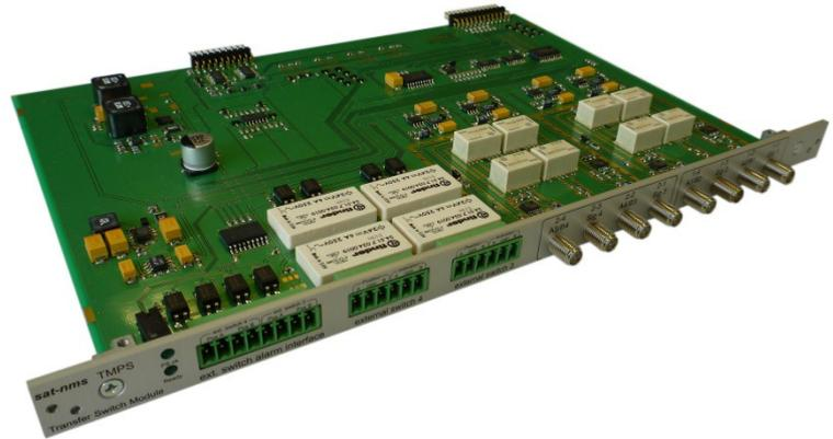
Each **sat-nms** TMPS module contains two latching transfer switches (DPDT). Each input is able to supply DC voltage to an LNB and performs monitoring of the input signal power. This enables the **sat-nms** TMPS to switch automatically in case of violation of the adjustable thresholds. Integrated on the same card are two waveguide switch driver outputs which are virtually connected to the transfer switches on the board. In addition 4 auxiliary inputs are integrated as external alarm inputs.
