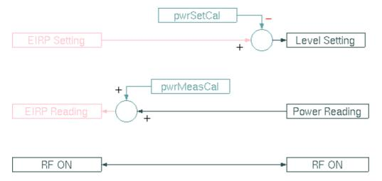
The diagram above illustrates the function of the Level-Set device. The device provides two calibrations offsets. One is used to translate an EIRP setting into a gain / output power setting to be applied at a device. The other offset translates a power reading into an EIRP value which is reported to the user. The RF-ON switch simply is routed through the device.
