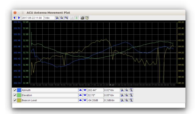
The window shows a diagram of the recorded tracking data, the fields and buttons in the tool bar permit to modify the appearance of the diagram as needed. Clicking into the diagram shows a marker which displays a readout of the value at the selected screen position in the status bar at the bottom of the screen.
