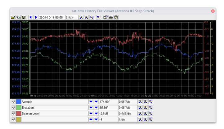
The window shows a diagram of the recorded data, the fields and buttons in the tool bar permit to modify the appearance of the diagram as needed. Clicking into the diagram shows a marker which displays a readout of the value at the selected screen position.
