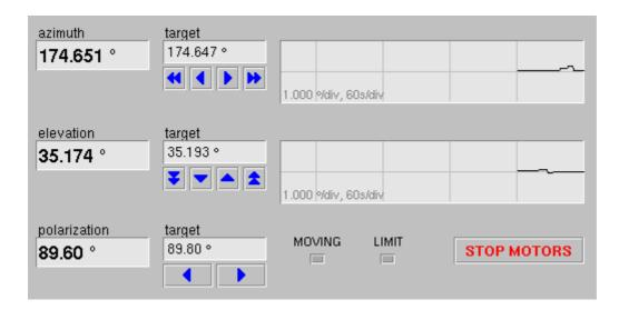
The fields labeled 'azimuth', 'elevation' and 'polarization' show the actual antenna pointing as read out from the angle encoders. For azimuth and elevation there is also a strip chart display of the angle. If you choose a high resolution scale for the chart, you can watch the antenna doing the tracking steps in the chart. Click with the right mouse button into the chart to get a pop-up menu for scales and other display options.
