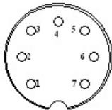
Connector type: Binder series 712, subminiature circular, connector (socket), front view
