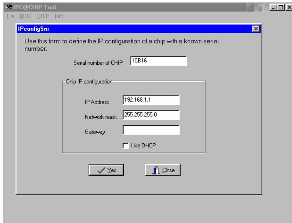
Now the IP configuration of the power sensor is completed. You may finally want to test if the power sensor is reachable now. Start your web browser and type the power sensor's IP address into the URL field of the browser. The power sensor should reply with it's main page, provided that the power sensor and your computer are configured for the same subnet.
