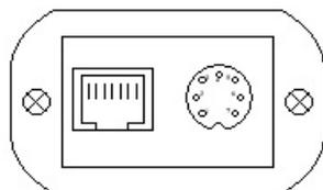
The RF input connector is a make N-type connector, mounted at one front panel of the power sensor enclosure. At the other side, the Ethernet and power supply connectors are mounted. The Ethernet connector is a standard 10 Base-T / RJ45 connector. Use a standard network cable to connect the power sensor to an Ethernet hub. If you want to connect your computer and the
