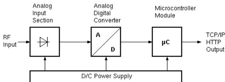
In the analog input section a microwave detector provides a DC voltage which is depending on the input power range either proportional to the input power or proportional to the input voltage of the input power at the power sensor. The relationship between input power level and the DC voltage to be measured in the last instance by the analog to digital converter is not necessarily to be known exactly, as this is measured and calibrated during the in-factory calibration of each individual sensor.
