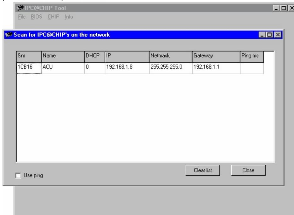
5. The serial number shown in the first column of the list, must match the serial number printed on the power sensor's enclosure. If the list stays empty, the power sensor is not connected properly. If there are more entries in the list, the configuration program has found other devices in this network segment which use the same technology.
