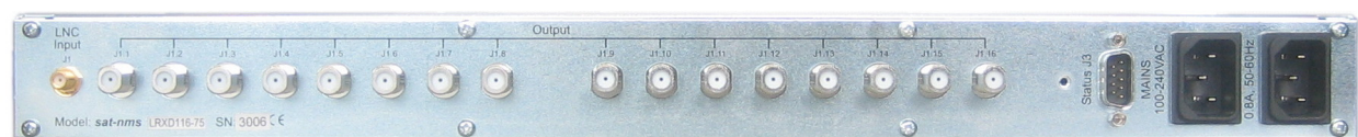
Rear Panel View of sat-nms LRXD116-75 with 1 SMA-Type Input Connectors and 16 F-Type Output Connectors
