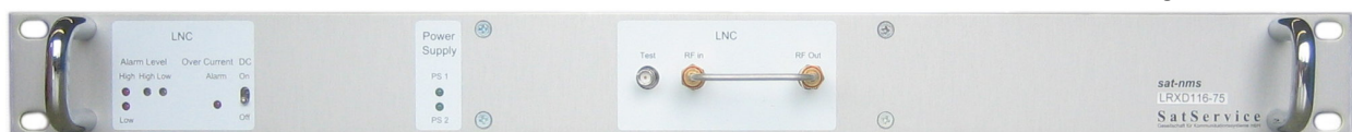
Front Panel View of sat-nms LRXD116-75 with Status LED's and Test Output
