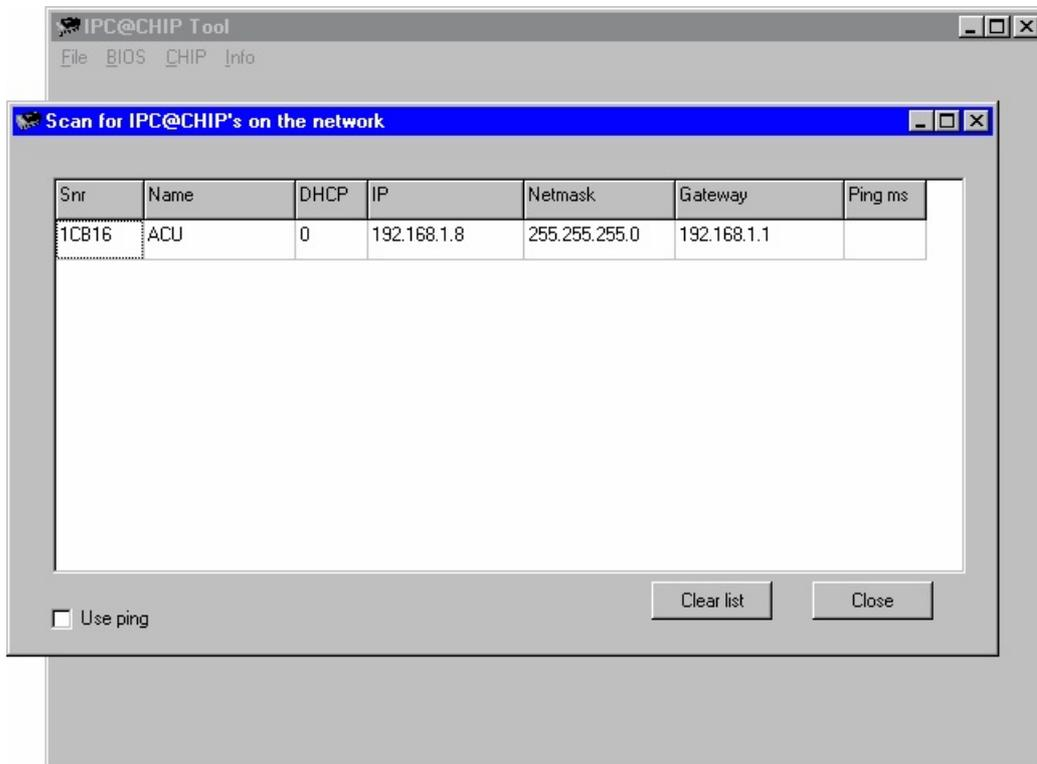
5. The serial number shown in the first column of the list, must match the serial number printed on the processor's enclosure. If the list stays empty, the DEICE-Controller is not connected properly. If there are more entries in the list, the configuration program has found other devices in this network segment which use the same technology.
