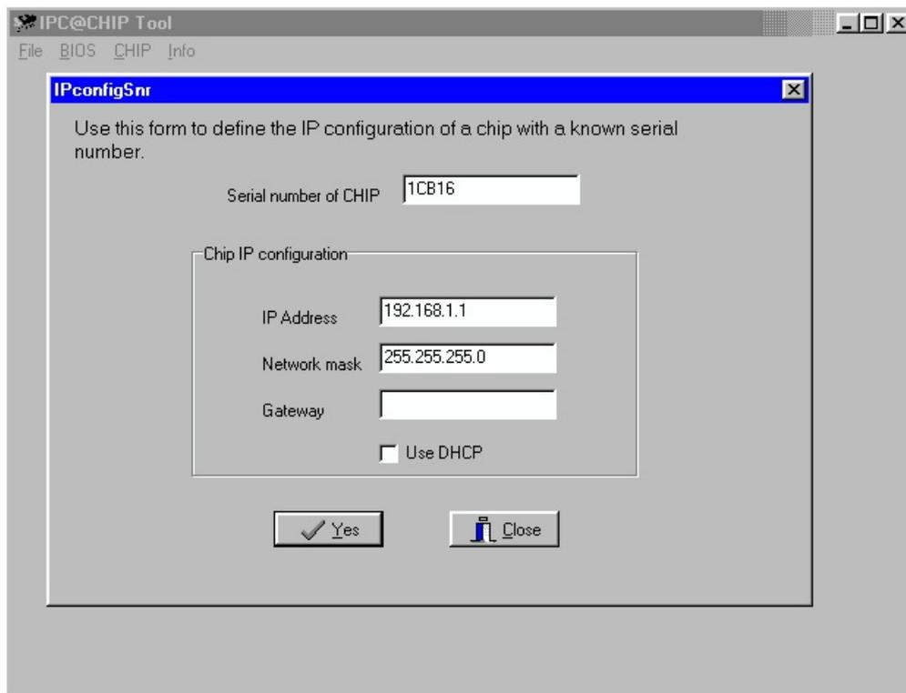
Now the IP configuration of the processor is completed. You may finally want to test if the DEICE-Controller is reachable now. Start your web browser and type the processor's IP address into the URL field of the browser. The DEICE-Controller should reply with its main page, provided that the processor and your computer are configured for the same subnet.
