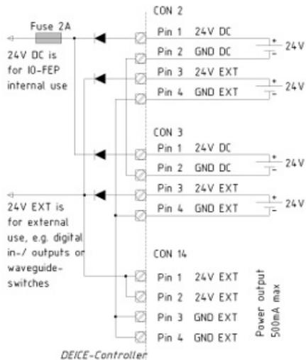
The power supply for the +24VDC circuit has to have a minimum current load of 150mA. The supply for the 24V\_EXT has to have a minimum current load of 500mA plus the current that will be taken from CON14 and the peak current of the biggest digital output to be controlled. Do not exceed the current-limit, in the circuit of 24V\_EXT is no fuse implemented! The maximum peak-current for switching the digital outputs is 5A.
